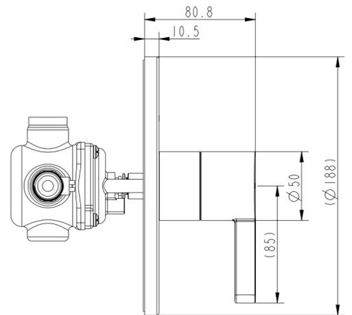
**Edge pressure balance valve trim kit, without-diverter**
